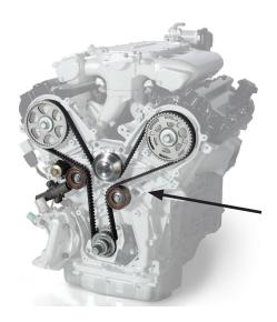
The shim is placed between the idler pulley and oil pump housing
